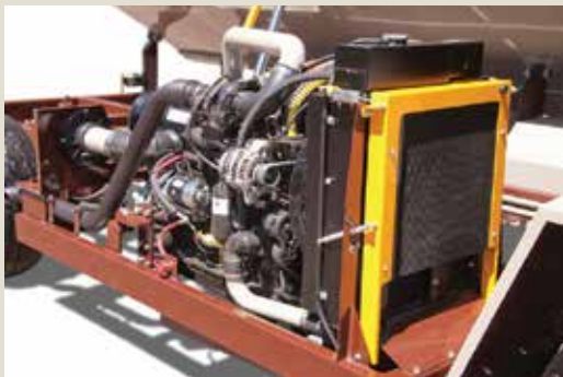
Cummins 4.5L, Tier 3, 110 H.P. Turbo Diesel Engine with easy access for service
