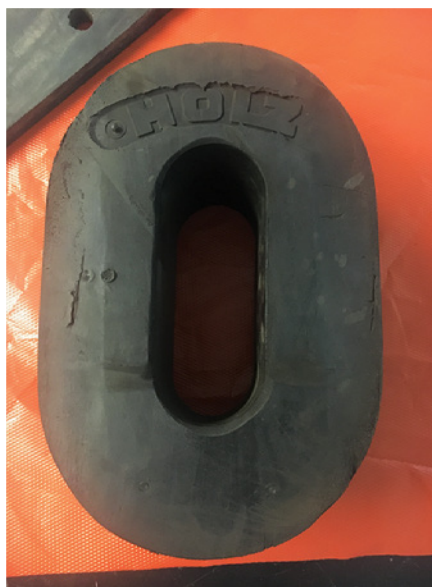
Top: When Wagner tested the TAS shaker pads during harvest, he found that while they performed well, they did generate slightly more heat than the control rubber shaker pads.
