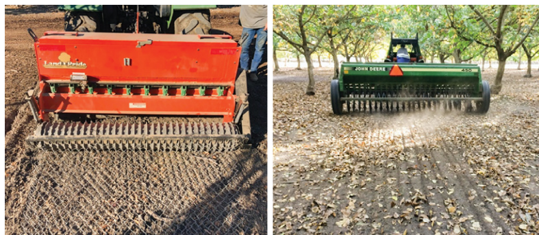
Photos: Left: the short and compact Land Pride PS15 Series has a chain link attached by the grower to help cover the seed once its set. Right: grain drills can also be used in the orchard if the bottom branches of the canopy will allow, and many times produce a wider planting width with one pass. Credit: Project Apis m.
